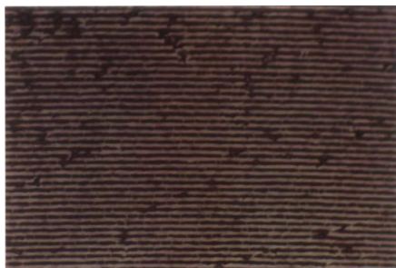
Figure 14. Photograph of the stripe texture exhibited by a mixture of BC12 and 8OCB, taken between rubbed glass plates. Reproduced with permission from (48); copyright © 2007 Europhysics Letters.
